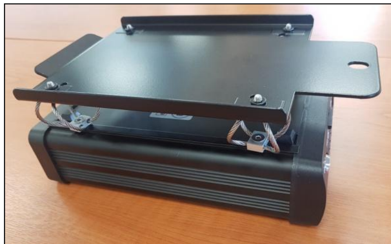
Figure 24 - Attaching the latching plate to the X300-16M
