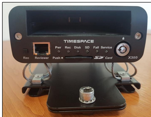
Figure 26 - X300-16M mounting plate screwed down
